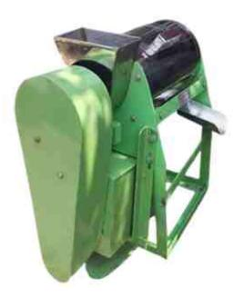
The machine has an infeed hopper from where the product is dumped into the pulper.
