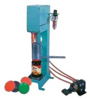
Pneumatic operated, equipped with pneumatic cylinder, provides constant pressure on the cap and then with gentle twist of handle the cap gets sealed. Air Compressor to be required for CC operating.
