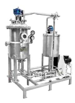
SUITABLE FOR COOKING AND CONCENTRATING PRODUCTS UNDER VACUUM EVAPORATED KETTLE.
